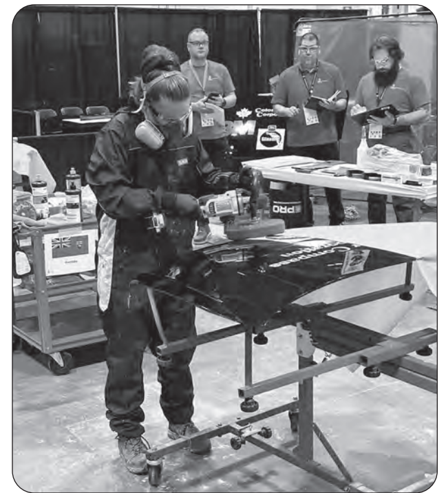
Cassandra Foy polishes imperfections from the surface of a vehicle hood as part of the refinishing process.
