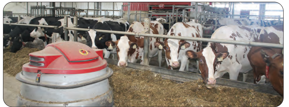
The automated feed pushers ensure food is in close reach for the cows.
